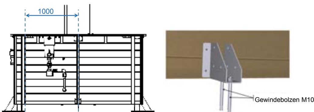
Abbildung 13 – a et b - Fitting the supporting brace shoes
